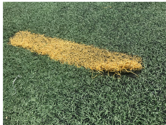
Figure 7 – Synthetic Turf Seam Failure
