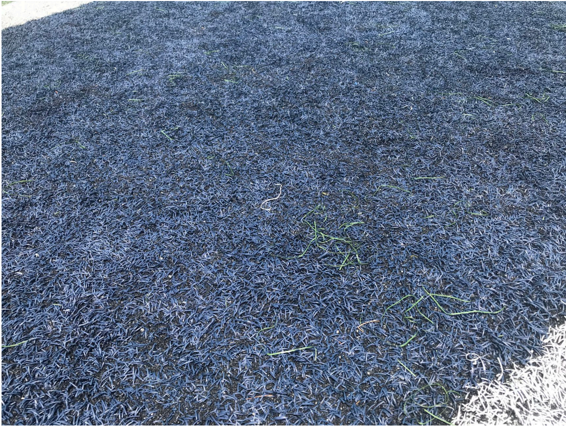
Figure 8 – Dislodged fibers are event throughout the field.
